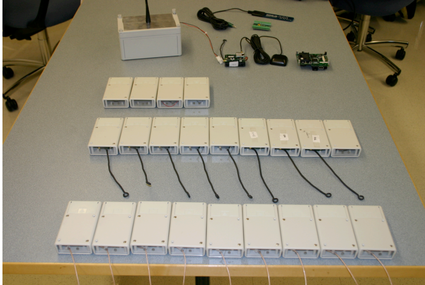
Mica2 Mote and Stargate Weather Packaging
