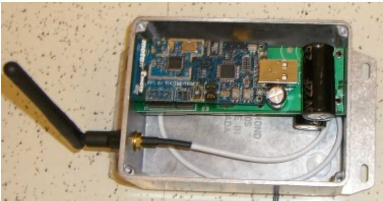
Figure 5: PCB and Mote mounted inside the enclosure
