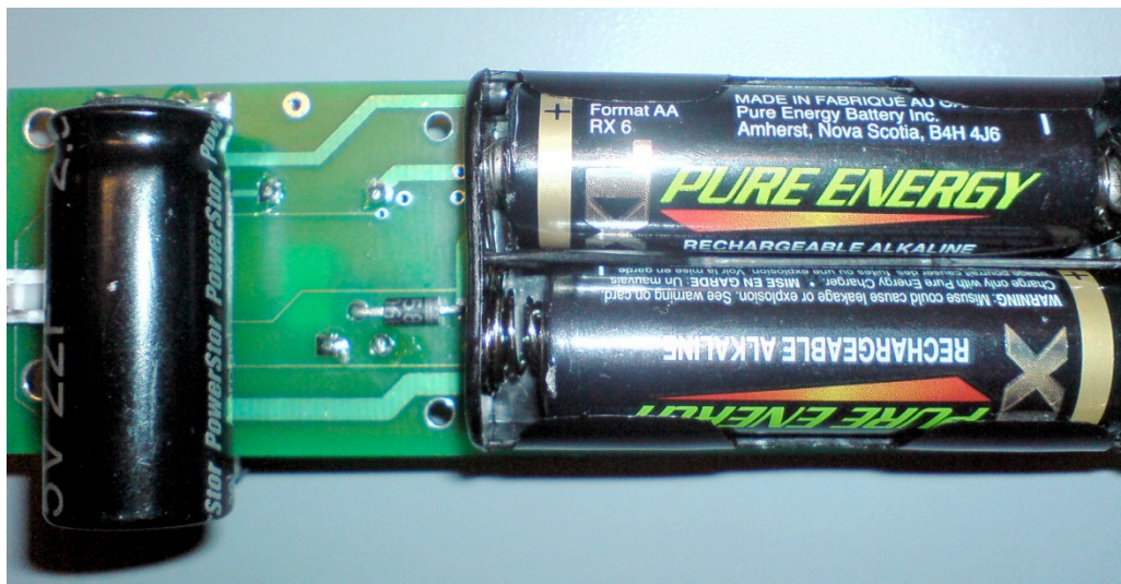
Figure 3: Back of the Printed Circuit Board that include second super capacitor the rechargeable batteries and the analog switches.
