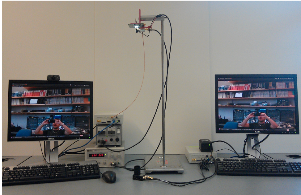
Figure 1: Real time video streaming from PC1 (left) to PC2 (right) over a 1m VLC link (center). The system is capable of transmitting over a distance of 3m.
